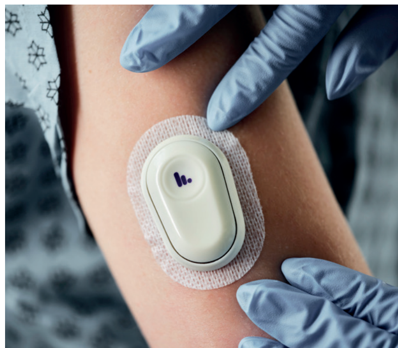
The Nutromics lab-on-a-patch uses biosensors and microneedles to provide real-time molecular monitoring
